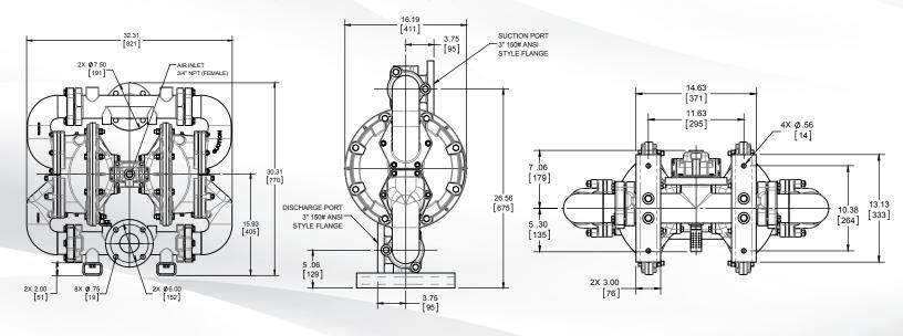
**HDF4-M Heavy Duty Flap Valve**Dimensions in inches (metric dimensions in brackets). Dimensional Tolerance .125" (3mm).
